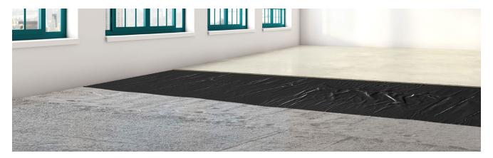
Part of the *TOPFLOW* liquid flowing screed range, *TOPFLOW* Screed A FINIO has been developed as a thin ready-mixed screed solution with minimal thickness of 15mm (Unbonded), 25mm (resilient layer - rubber based resilient layers only) 30mm (floating insulationmust be a minimum 140KPa), if not depths must be increased to 35mm domestic, 40mm commercial.
