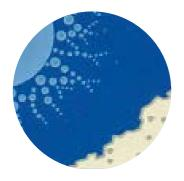
Crystals produced by the hydration reaction grow away from each cement particle during curing.
