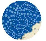
Finer, stronger hydration crystals develop during the curing process.
